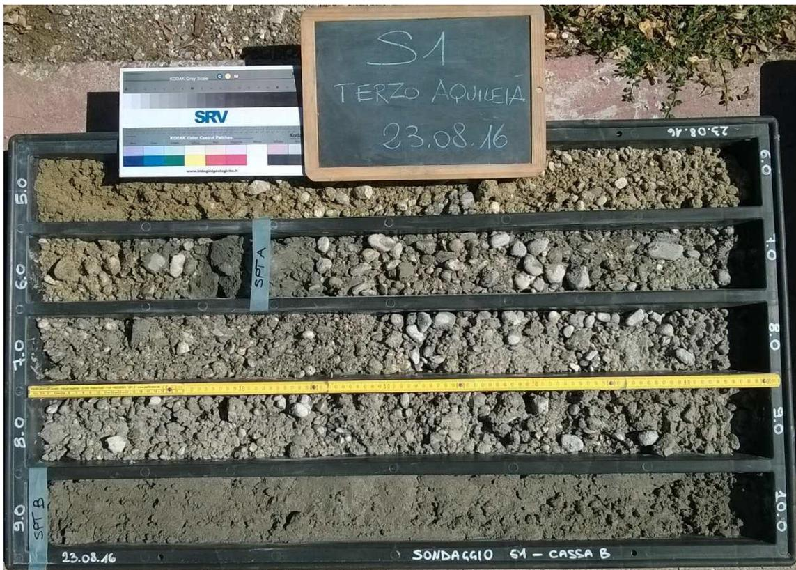
FOTO N° 2: SONDAGGIO S1, CASSETTA B: DA 5.0 A 10.0 METRI
